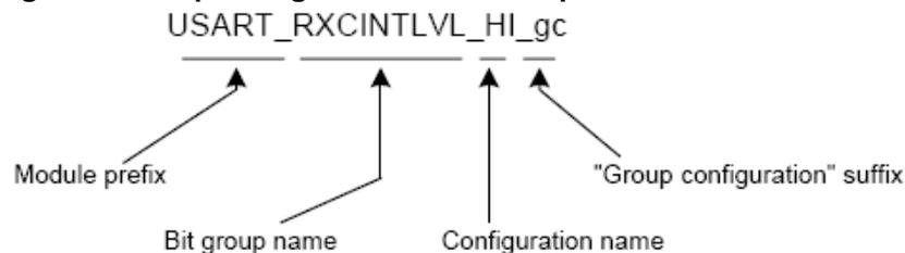
From Figure 2 one can see that the group configuration is used for the Receive complete interrupt level (RXCINTLVL) bits in a USART module. This specific group configuration selects a high (HI) interrupt level.
