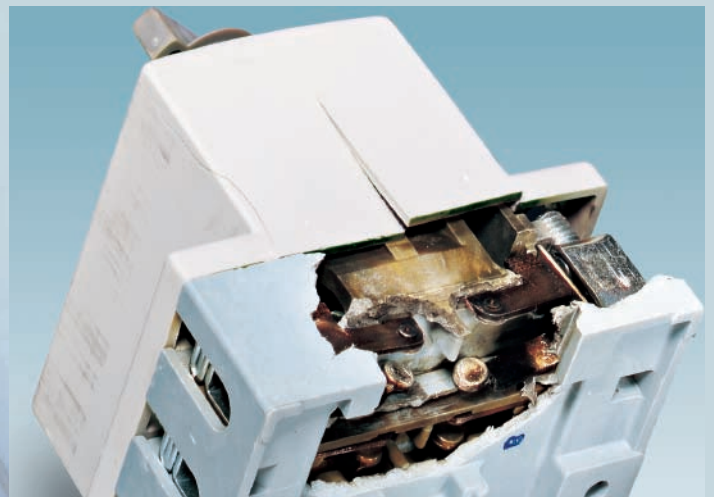
Fig. 1b: Destroyed residual current circuit breaker (RCD)
