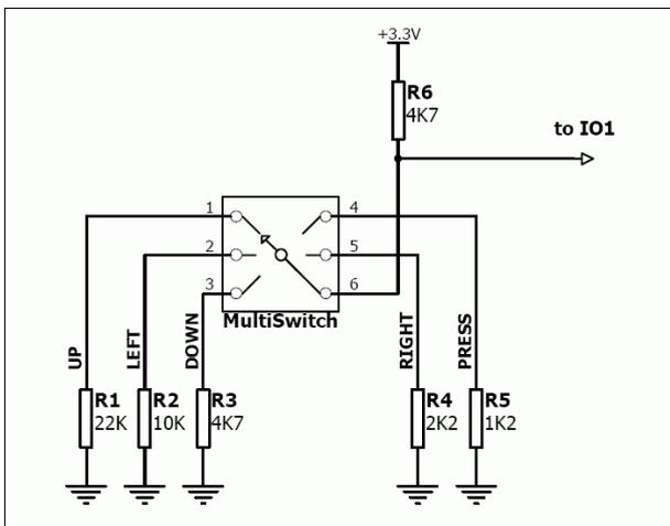
Unused buttons do not need resistors to be connected to the circuit. The table below lists the buttons and corresponding resistor values.
