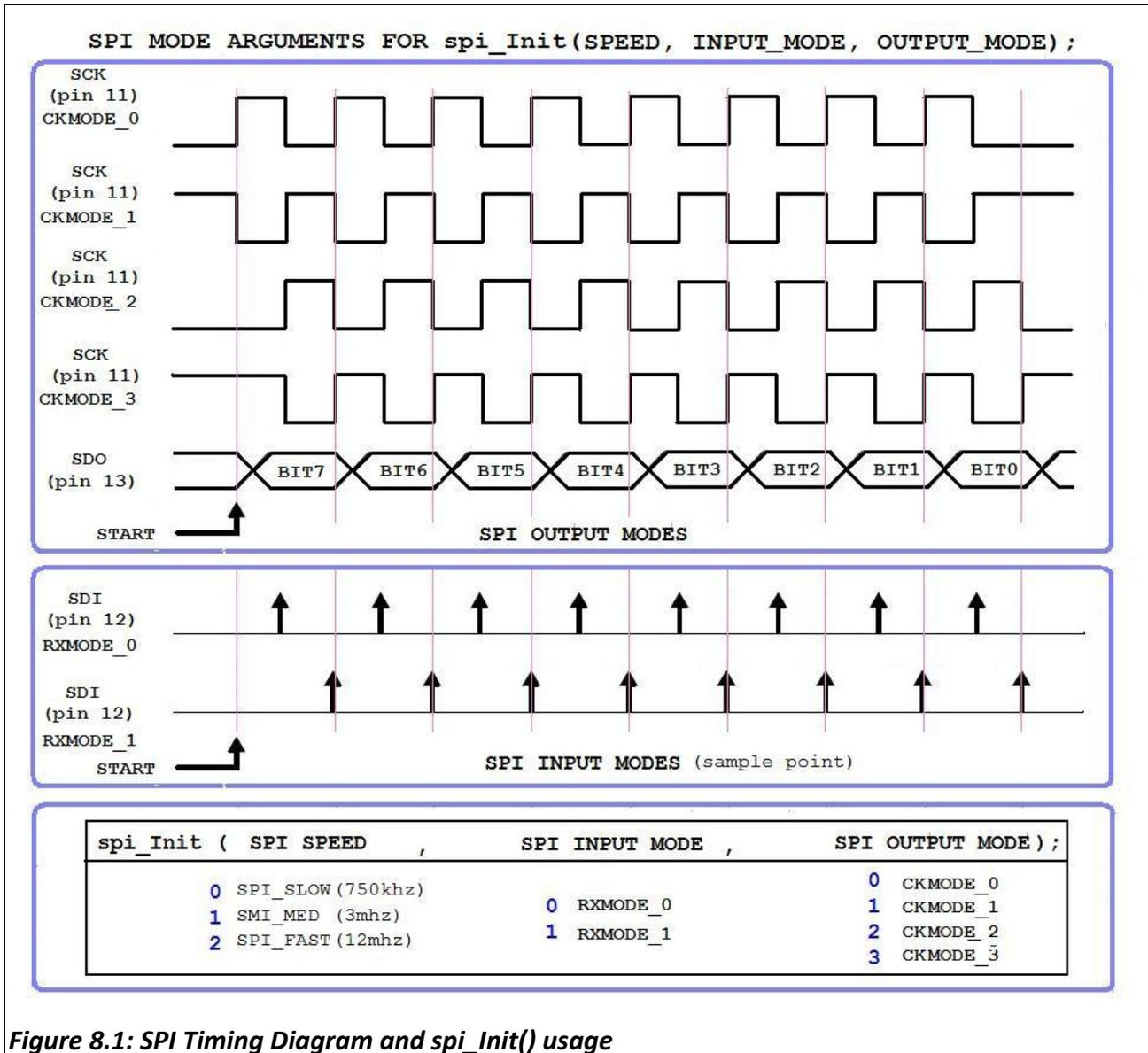
**Figure 8.1: SPI Timing Diagram and `spi_Init()` usage**
