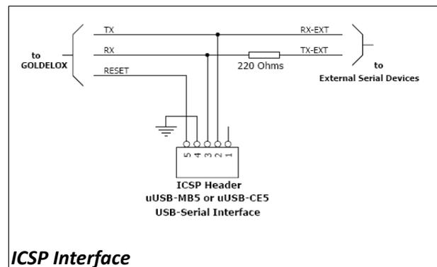
The PmmC file is programmed into the device with the aid of "**PmmC Loader**", a PC based software tool. To provide a link between the PC and the ICSP interface a USB to Serial converter is required. A range of custom made micro-USB devices such as the uUSB-MB5 and the uUSB-CE5 are available from 4D Systems. For further details refer to '**Section 6: Development and Support Tools**'.
