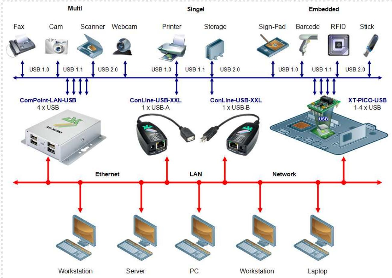
Then they can be directly addressed and controlled via a PC in the network. A driver is installed on the PC which makes you available such USB devices via a virtual USB interface. By disconnecting the virtual connection in the software such USB devices can also be shared in the network and in this way they are available from any place.
