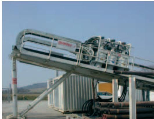
The hardliner. For all applications not allowing the use of a plastic chain, for example in steel works, foundries, on machine tools and oil-rigs. Made of galvanized steel with drilled aluminium frames or steel separators (adjustable separators). Available in stainless steel AISI 316 if required.
