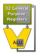
Central in the AVR architecture is the fast-access register file with 32  $\times$  8-bit general purpose working registers directly connected to the Arithmetic Logic Unit. Within a single clock cycle the ALU can be fed two arbitrary registers, do a requested operation, and write back the result.
