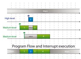
A second interrupt at an interrupt level already being serviced, will pend until the first interrupt routine finishes.
