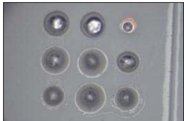
Fig. 7: Unfilled thermal vias show solder wicking, if they are used in solder pads
