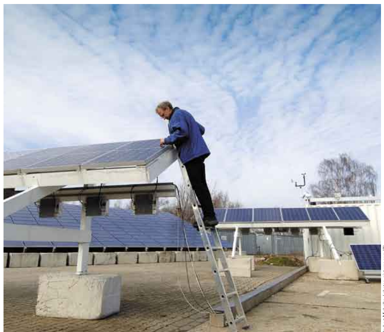
Measurements in the PHOTON laboratory: the STC-output of a module is determined by the flasher within a split second. The measurement of the yield will take a little longer – namely, one year on the free-field test facility.
