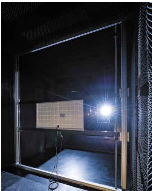
Measurements in the PHOTON laboratory: the STC-output of a module is determined by the flasher within a split second. The measurement of the yield will take a little longer – namely, one year on the free-field test facility.
