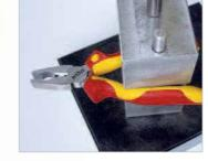
Pressure tests No disruptive discharge may occur at a pressure load of 20 N, a temperature of 70° C and a test voltage of 5,000 V AC.
