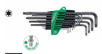
366R SZ13 TORX<sup>®</sup> MagicSpring<sup>®</sup> L-key set in ProStar holder, 13-pcs. Retaining spring holds TORX<sup>®</sup> screws in place. Blade: Chrome-vanadium steel, through hardened, manganese-phosphated. Application: For setting and tightening TORX<sup>®</sup> screws in difficult to access areas. Makes simple removal of each individual key possible Extra: without movement of the others.
