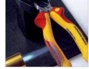
Testing the combustion behaviour A flame is pointed at the tool for ten seconds. The insulating material may then not continue to burn, but instead must extinguish.
