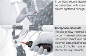
Composite materials The use of new materials such as carbon make using torque tools vital. The carbon structure is damaged by the incorrect torque during fastening. Because of this, the material no longer withstands the requirements.
