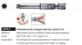
specially in difficult to access areas. Extra: MagicRing<sup>®</sup> made from spring steel holds all standard screws in every position. Ball end allows a working angle up to 25°.
