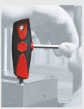
A tool that is a pleasure to use. Using the side blade for even areater toraue. a supporting hand stabilises the handle and prevents the blade from slipping.
