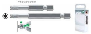
TORX<sup>®</sup> ball end bits 50 mm, in plastic box. Plastic box, reusable and dust repellent. Easily identifiable content with large symbols. The TORX® ball end enables fastening and unfastening at an angle of up to 25°. With elongated TORX® profile behind ball end.
