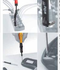
Circular plug connector protection class IP67 For correct functioning of distributions systems on machines, the correct torque must be observed when connecting the circular plug connectors. Otherwise the protection class IP67 cannot be complied
