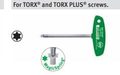
TORX<sup>®</sup> driver with T-handle. 364R With MagicSpring<sup>®</sup>. Blade: Chrome-vanadium steel, through hardened, chrome-plated. Handle: Wiha Classic T-handle. Application: For high torque transfer with minimal effort. MagicSpring® made of stainless steel holds TORX® screws Extra: tight at various angles. ChromTop® blade tip for the highest accuracy Blade made of hexagonal material is particularly capable of withstanding stress.
