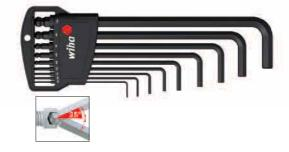
369 H9B Hexagon ball end L-key set in Classic holder. Manganese-phosphated, 9 pcs. Blade: Chrome-vanadium steel, through hardened, manganese-phosphated. Standards: Based on ISO 2936L. Application: Especially for screws that are difficult to access. Extra: Popular key sizes kept in a well-organised holder. Simple, rapid operation with solid stopping point for L-keys. The ball end enables the user to work at angles up to 25°.
