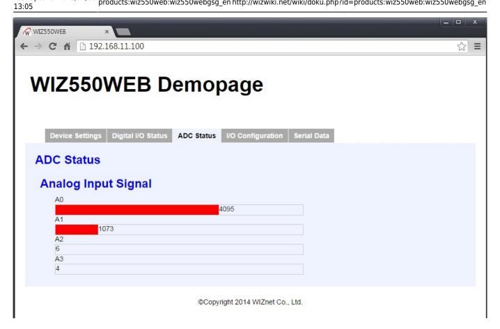
The Analog input signal through ADC changes into a bar graphs is displayed in real-time.
