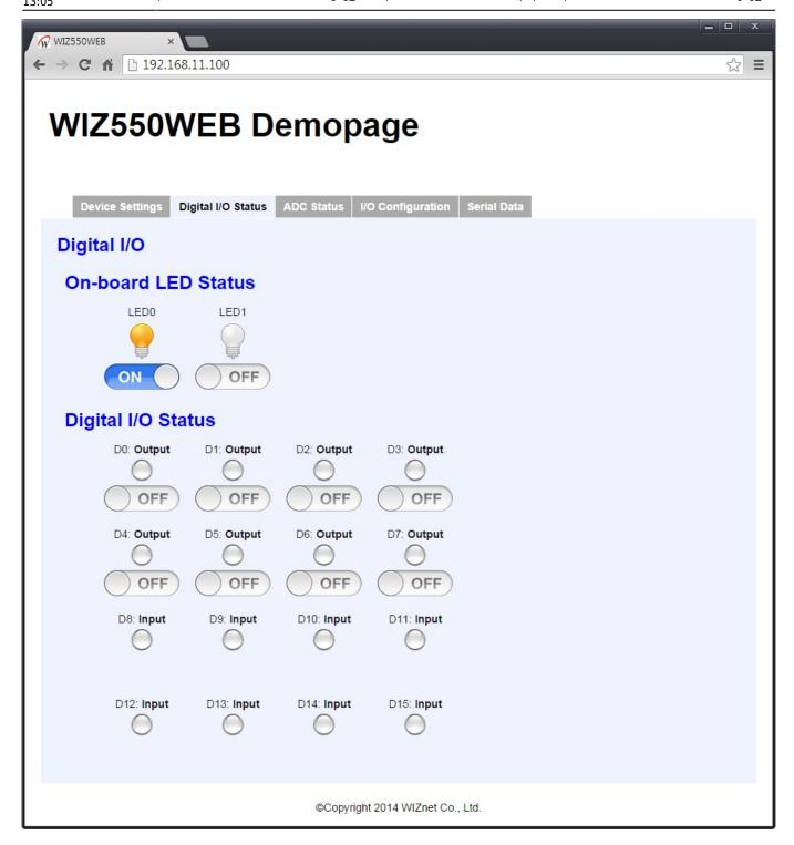
[On-board LED] WIZ550web's LEDs can be control by On/Off button in web page. [Digital I/O Status] Digital I/O Status indicates the current status. When the I/O is output, users can set On/Off. Each I/O information are configured as below.
