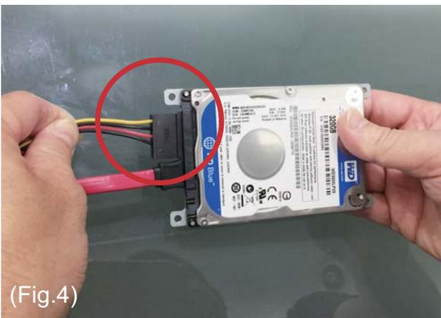
4. Connect the SATA Power cable with HDD. (Fig.4)
