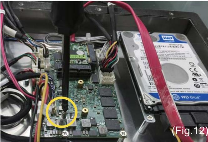
12. Unscrew the (M2\*6) screw from the screw thread on motherboard. (Fig.12)
