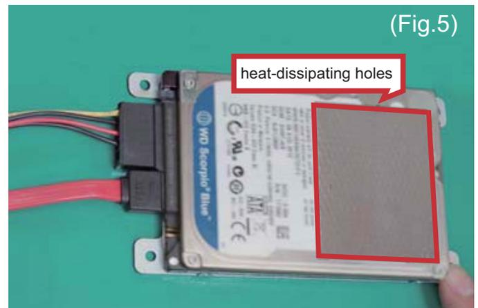
5. Attach the thermal pad on the HDD and avoid the heat-dissipating holes at the same time. (Fig.5)
