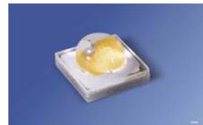
**Small size high-flux LED for slim designs (between 200 mA and 1.5 A constant current). 278 lm and 126 lm/W at 700 mA; 152 lm and 146 lm/W at 350 mA.**
