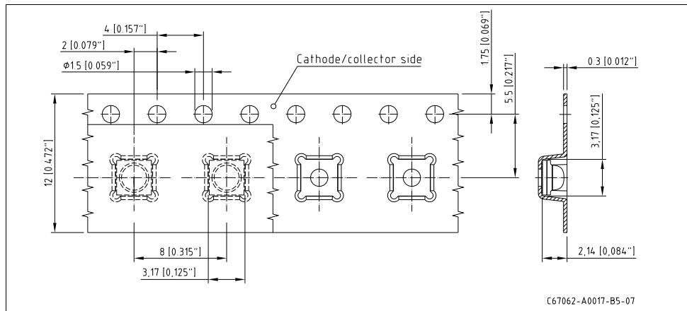
**Tape and Reel<sup>5)</sup> page 20****Gurtverpackung<sup>5)</sup> Seite 20**12 mm tape with 600 pcs. on  $\varnothing 180$  mm
